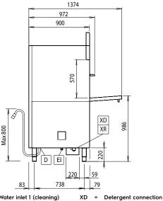
Cold Water inlet 1 (cleaning) Drain
